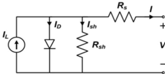
Figure 2 Single Diode model for solar
