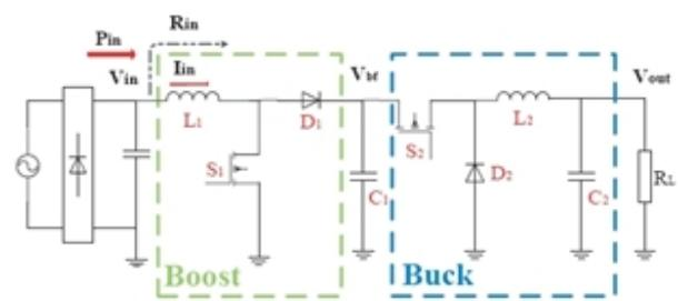
Figure 3 Cascaded Boost- Buck converter [5]
