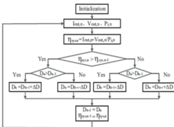
Figure 4 Flowchart of the P&O-based tracking [6]
